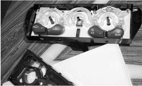
Above: Photo 5. View beneath the Control Head face plate.
