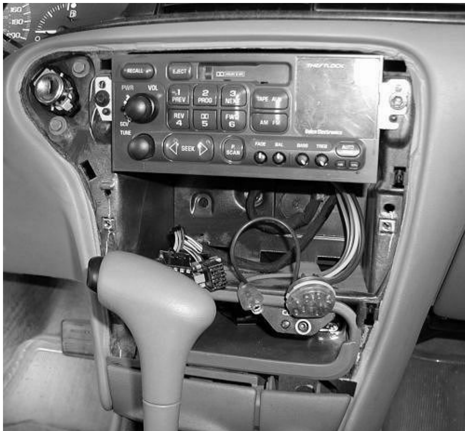
Above: Photo 1. 1997 Malibu panel with the Control Head and bezel removed.
